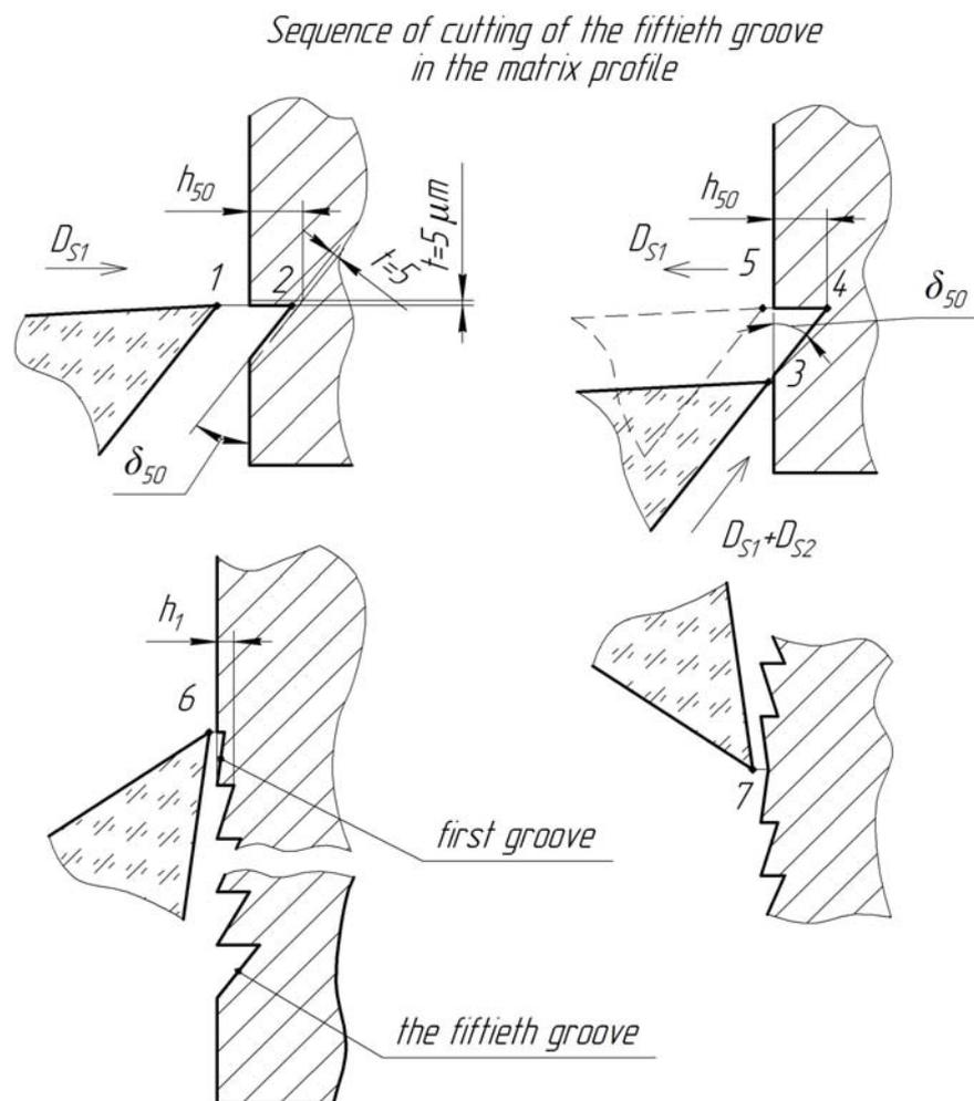
**Figure 5.** Cutting sequence of the matrix profiles for Fresnel lenses
