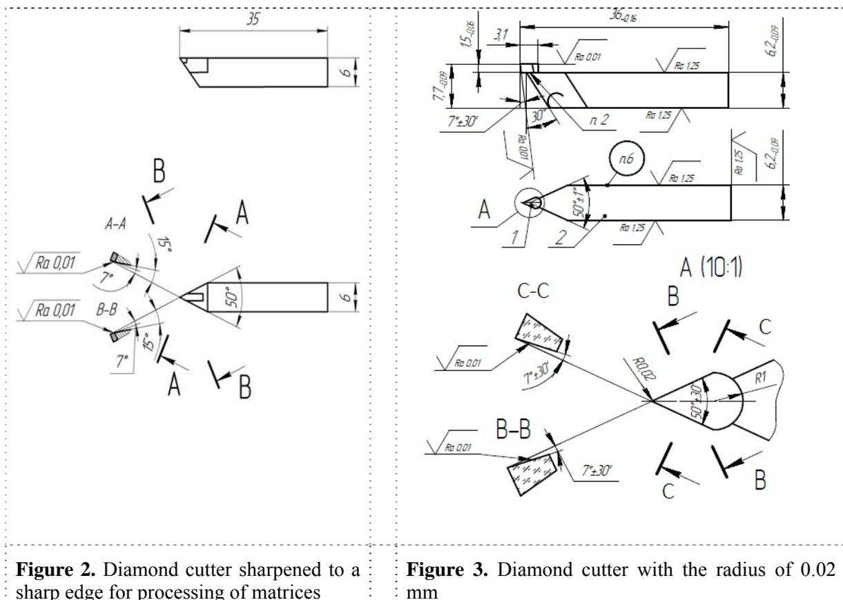
**Figure 2.** Diamond cutter sharpened to a sharp edge for processing of matrices
